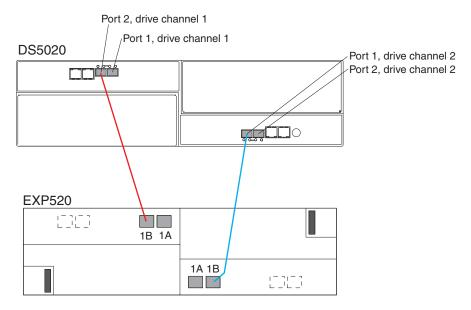
Figure 46. Cabling for one DS5020 and one EXP520 storage expansion enclosure
